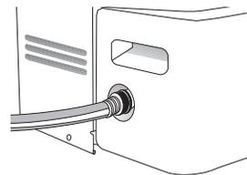
3. Attach a garden hose to drain hose connector. The garden hose should not be longer than 8 ft (2.4 m). Run other end of garden hose into a floor drain. Check that the hose lies flat and in the drain.
