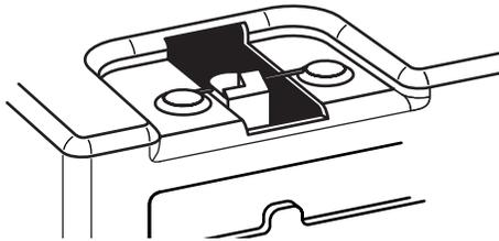
You can set the adjustable Water Level Float at the "high" or "low" position. Both settings will turn off the dehumidifier automatically. To adjust water level, push float left or right until it snaps into place.
