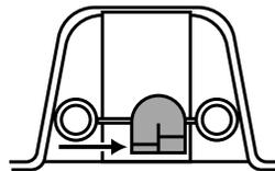
"Low" setting: Slide Water Level Float to "low" position - right side of opening - to make the bucket lighter to carry. The dehumidifier will shut off automatically when bucket is  $\frac{1}{2}$  full.
