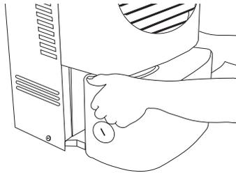
1. Use both side handles to lift bucket. Pull bucket forward and remove.
