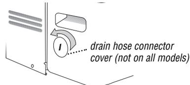
1. If your dehumidifier does not have a drain hose connector cover, go to Step 2.
