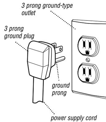
For your personal safety, this dehumidifier must be grounded. This dehumidifier is equipped with a power supply cord having a 3 prong ground plug.
