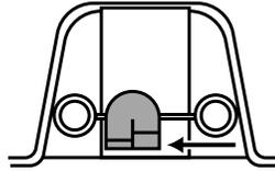
"High" setting: Water Level Float is preset to the "high" position - left side of opening. The dehumidifier will shut off automatically when bucket is  $\frac{3}{4}$  full.
