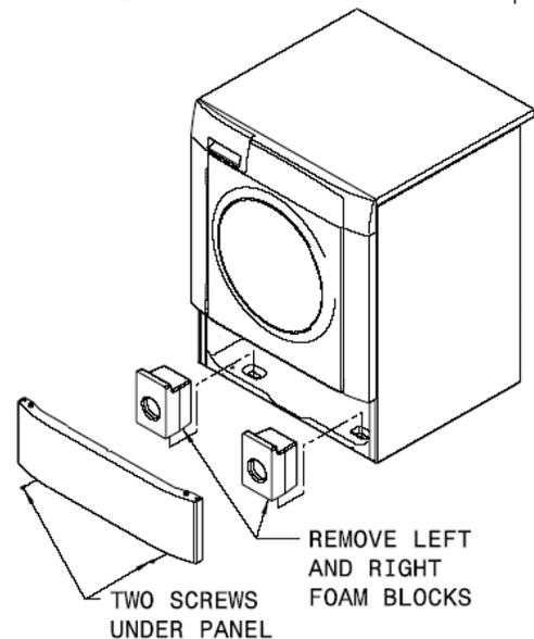
11. Remove the two (2) styrofoam blocks located under the drum (a yellow ribbon surrounds the items to be removed). Lift up on the drum, tilt the base of the foam blocks inwards toward the rear of the washer until free, then pull them out.
