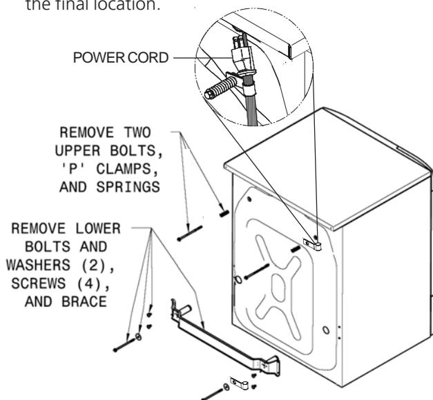
6. Remove the following from the back panel of the washer: 4 packaging bolts, 2 packaging springs, 2 washers, 2 metal "P" clamps, 4 screws, 1 packaging brace.
