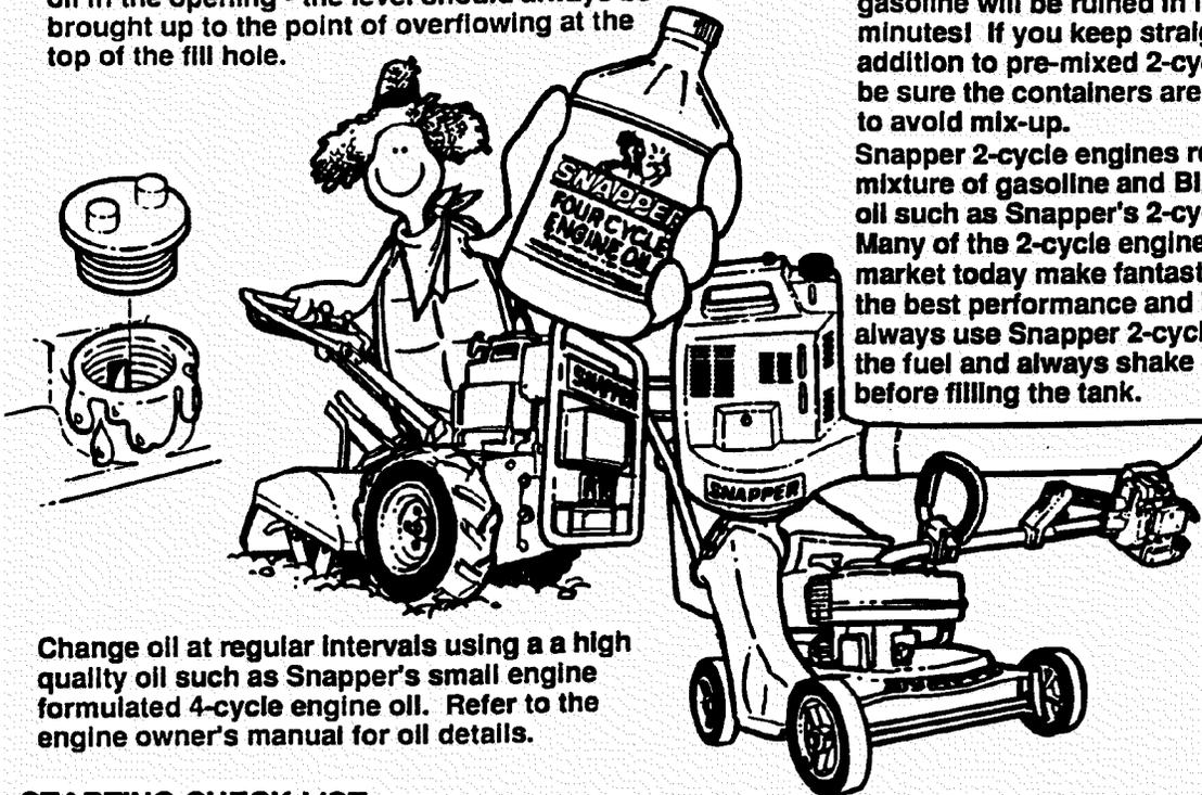
On 2-cycle engines, lubrication must be provided by an exact mixture of gasoline and 2-cycle air-cooled engine oil. A 2-cycle engine that is mistakenly run on straight gasoline will be ruined in less than 5 minutes! If you keep straight gasoline in addition to pre-mixed 2-cycle engine fuel, be sure the containers are clearly marked to avoid mix-up.
